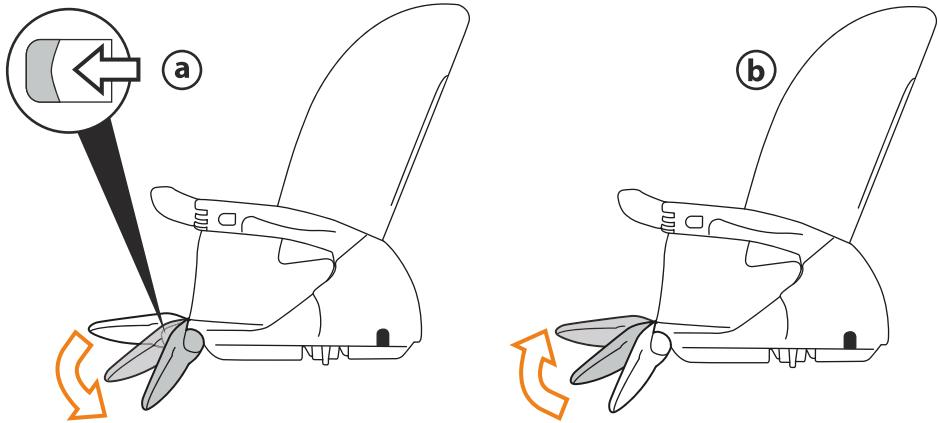
11 FOOTREST: To lower the footrest push the two levers downwards and then push the footrest downwards (fig\_a), to raise the footrest lift it upwards (fig\_b).
