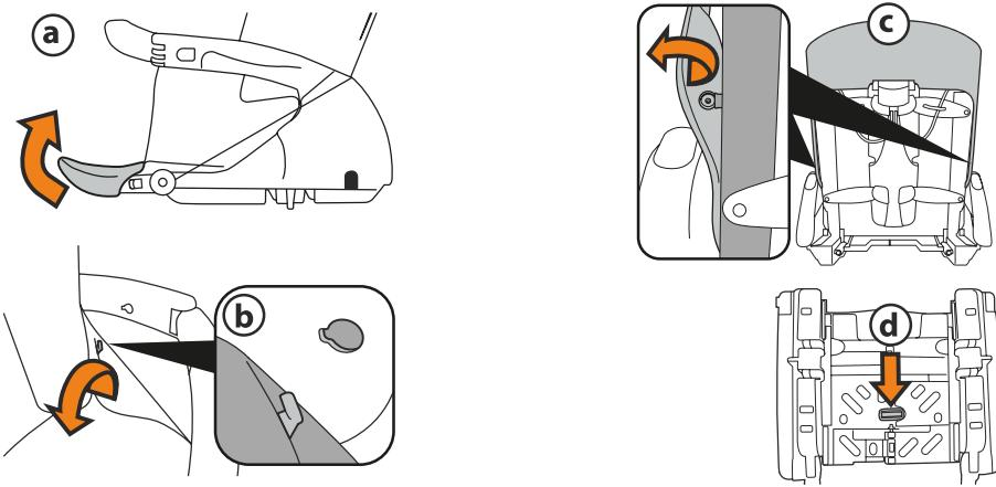
**21 REMOVABLE COVERS:** Pull the fabric covering off the ledge (fig\_a), release the attachments of the fabric covering from the armrests (fig\_b), unfasten the buttons on the sides of the backrest (fig\_c) and remove the leg divider strap from above by pushing it from under the seat (fig\_d).
