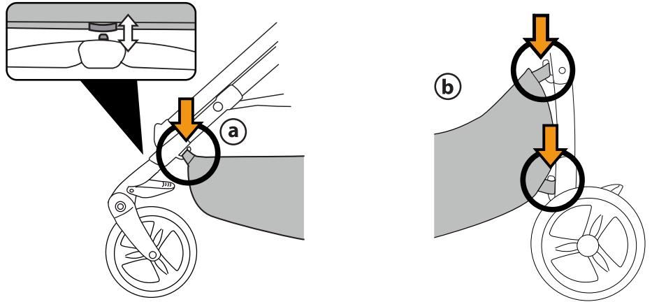
**2 FITTING THE BASKET:** Slip the loops onto the hooks at the front (fig\_a) and the rear (fig\_b).
