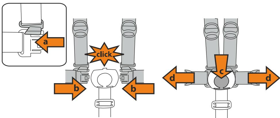
12 FIVE POINT SAFETY HARNESS: To fasten it, push the two waist strap buckles (with the shoulder straps attached arrow\_a) into the leg divider until they click into place (arrow\_b). To unfasten it, press the round button in the centre of the buckle (arrow\_c) and pull the waist straps out (arrow\_d).
