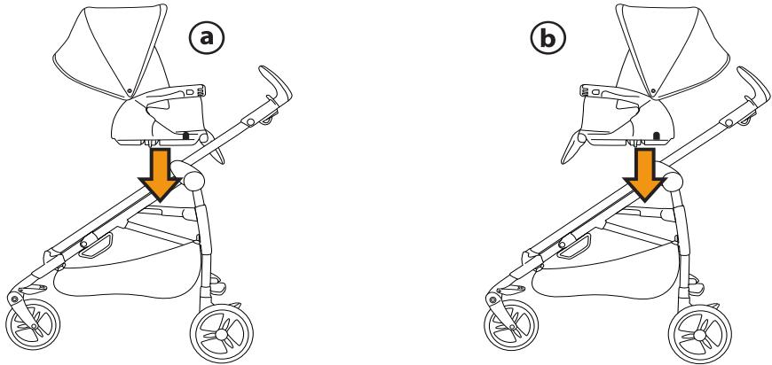
**7 MOUNTING THE SEAT TO THE CHASSIS:** the reversible seat can be attached to the chassis either facing the person pushing the stroller (fig\_a), or facing forwards (fig\_b), place the seat on the chassis so that it is aligned with the relative symbols and press downwards with both hands until you hear two clicks confirming that it has locked into position. Ensure the seat is correctly secured by attempting to pull it upwards by gripping the front bar.
