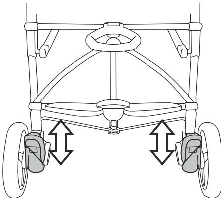
**6 BRAKES:** Press a brake lever to immobilize the chassis (fig\_a) and lift the lever to release it (fig\_b).
