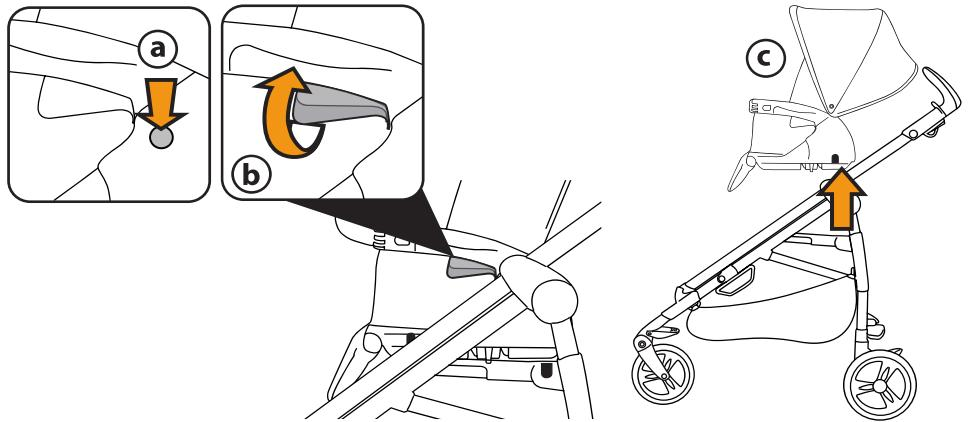
**8 REMOVING THE SEAT FROM THE CHASSIS:** Press the two levers under the armrests (fig\_a) and pull up the seat (fig\_b) until it is released. The seat can be removed from and re-attached to the chassis when there is a child in it.
