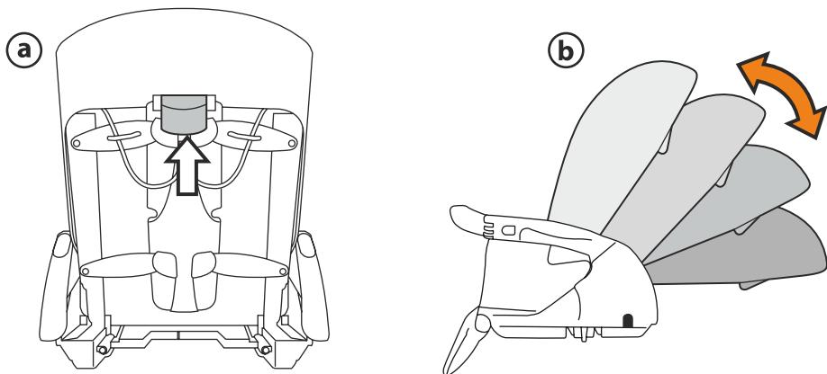
**10 BACKREST:** To recline the backrest lift the lever (fig\_a) and choose one of the 4 positions (fig\_b).
