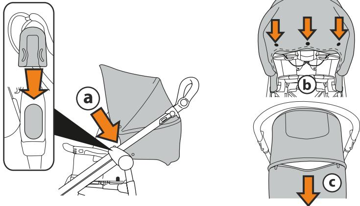
15 HOOD: to attach the hood insert the connections into the sides of the seat (fig\_a) and then fasten the buttons on the rear of the backrest (fig\_b). To remove the hood: disengage the connections and unbutton from the backrest. To raise the hood: pull it towards you, to close the hood: push it back. To convert the hood into a sun canopy, open the double zipper (fig\_c) and unfasten the buttons on the rear of the backrest.
