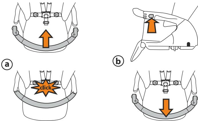
**9 FRONT BAR:** To attach the front bar, guide the connections into the armrests and push towards the seat until they click into place (fig\_a). To remove the front bar, press the two buttons and pull it out (fig\_b). To make it easier for the child to get in and out, it is possible to open the front bar on one side only. If you wish to use the stroller without the front bar, put the caps back in the armrests.
