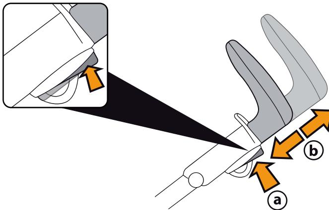
4 ADJUSTABLE HANDLES: To raise or lower the handles hold the button down (fig\_a) and adjust them (fig\_b).
