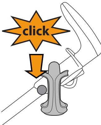
3 FITTING THE CUP HOLDER: insert the cup holder on the corresponding peg and press down until it clicks into place (fig\_a).
