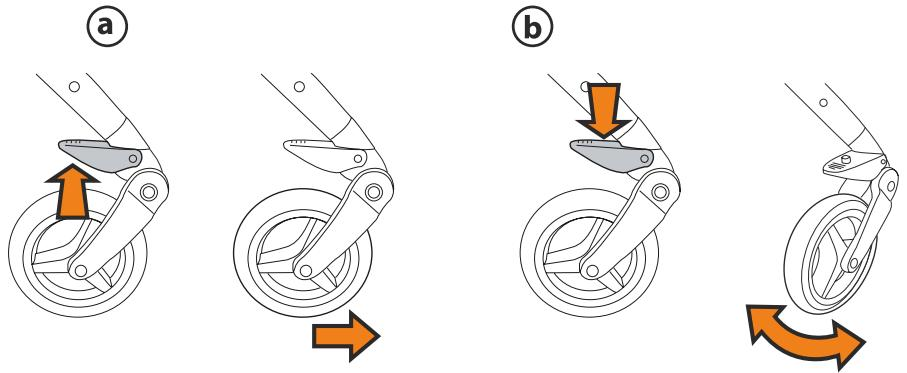
**5 FIXED OR SWIVELLING FRONT WHEELS:** Lift the levers to prevent the wheels from swiveling (fig\_a) and lower them to allow the wheels to swivel (fig\_b). On uneven surfaces, the wheels should be set to their fixed position.
