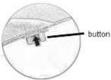
4.To assemble/disassemble the front bumper bar: align front bumper pegs with the holes on bumper adaptors, slide and press into unit hear "clicks", press down both buttons to disassemble bumper from adaptors
