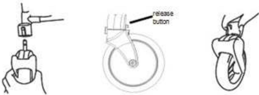
2.To assemble/disassemble front wheels: make the parts of the front wheels inserted in the support, the block flipping out. Press the block pull the front wheels out,the wheels removed
