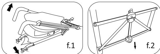
**How to assemble/disassemble front wheels:**
